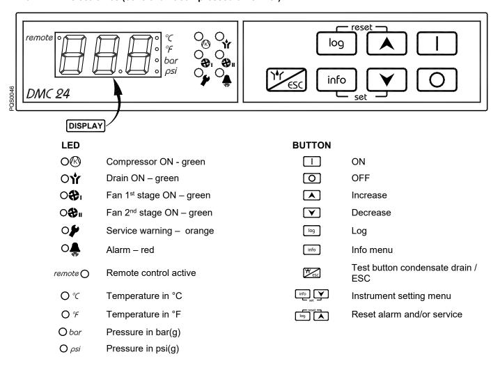
The DMC24 controls all operations, alarms and instrument settings of the chiller. The display and the LEDs indicate all operating conditions.
