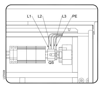
A residual-current device (RCD) with  $I\Delta n=0.03A$  is suggested. The cross-section of the power supply cables must correspond to the consumption of the chiller. In this respect, the ambient temperature, the cable laying conditions, the length of the cables and the requirements of the local electricity supplier need to be considered.
