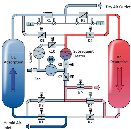
check valve **R1**, exiting to the air distribution system. The adsorption phase ends based on either the time or outlet pressure dew point (option).
