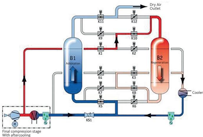
The whole procedure is executed with operating pressure, not only in the adsorption stage but also in the regeneration and cooling stages. This therefore enables the resulting compression heat to be utilized for regeneration for oil-free compressors for pressurized air.
