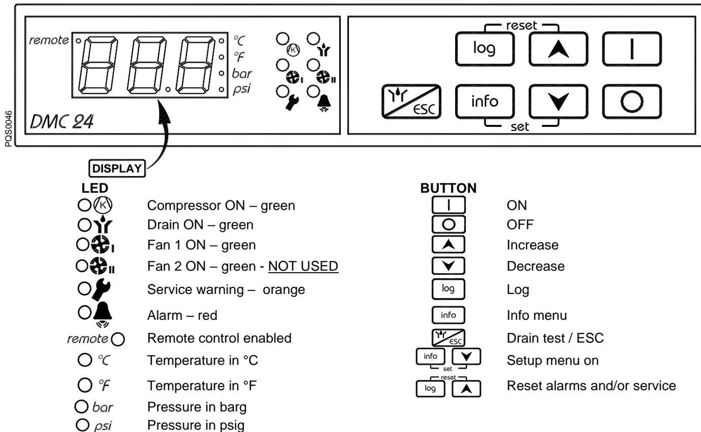
The DMC24 controls all operations, alarms and instrument settings of the dryer. The display and the LEDs indicate all operating conditions.
