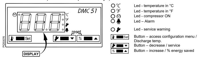
The DMC51 controls all the operations, alarms and dryer operation set-up.
