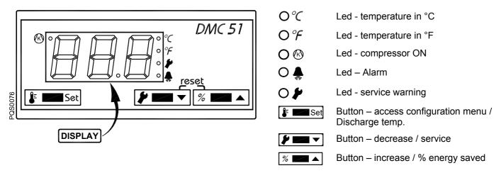
The DMC51 controls all the operations, alarms and dryer operation set-up.
