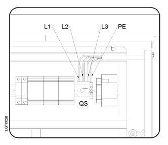
A residual-current device (RCD) with  $I\Delta n = 0.3A$  Class B is suggested. The cross section of the power supply cables must comply with the consumption of the dryer, while keeping into account also the ambient temperature, the conditions of the mains installation, the length of the cables, and the requirements enforced by the local Power Provider.
