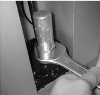
2. Disconnect silencer from valve block.
