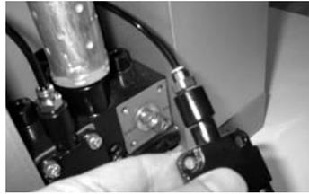
5. Disconnect tubing from fitting on bonnet.
