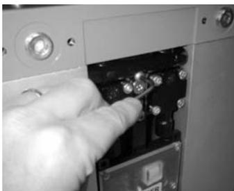
5. After thoroughly drying purge plug, push back into port in valve block. Ensure that 'o' rings are in place and in good condition.
