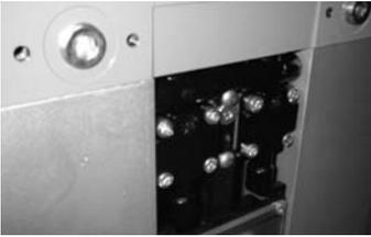
1. Remove front panel as described in §11.5 and locate position of upper and lower bonnets.
