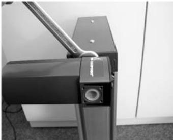
3. Inlet filter is fitted to dryer in vertical orientation. Tighten fitting.
