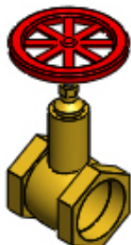
Rendered drawing of purge flow control valve
