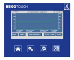
Pressing **HISTOGRAM** allow a real time trend line of the relative humidity of the dryer. At full a total of 80 minutes can be displayed.
