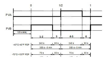
The cycle time is factory set for operation at 100 psig inlet air pressure and 100 °F inlet air temperature.
