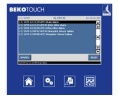
The controller has ability to continually monitor specific dryer characteristics along with any ancillary equipment provided it is connected to the controller. If there is a functional issue associated with normal operation, an alarm will be triggered and the pop-up ribbon will be displayed on the bottom of the active screen. The alarm types are listed below:
