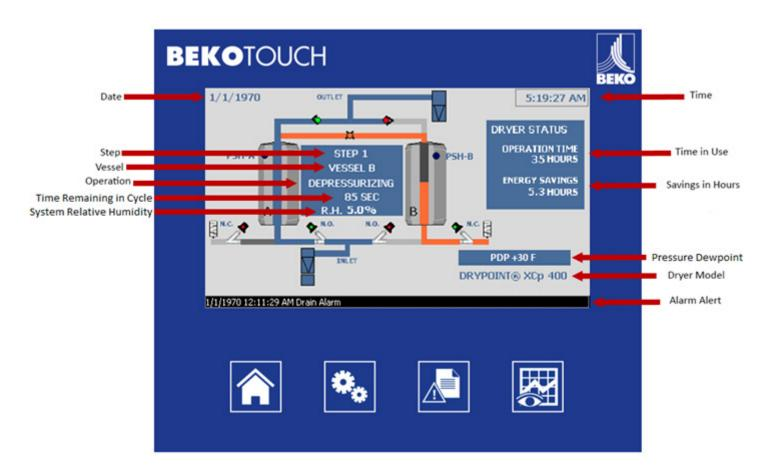
Here, the controller provides the system information along with an animation of the drying process based on the operating sequence it is on. Each step is detailed below along with a screen shot of the process.
