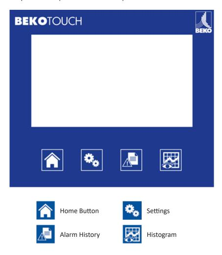
The operation of the dryer is controlled and monitored constantly by the advanced system controller. This is a multifunction device:
