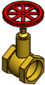
Rendered drawing of purge flow control valve
