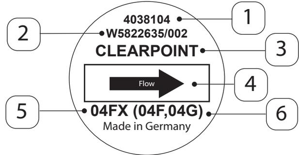
Filter element sticker - view of filter element base
