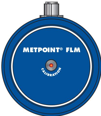
The METPOINT® FLM features a LED calibration indicator mounted at the top of the housing. After 15 months, the LED begins to flash, indicating that the device needs to be calibrated. The flashing LED does not have any effect on the measuring process, and the device continues to provide accurate measuring signals.
