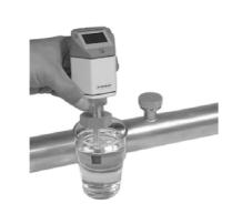
The sensor can be cleaned by carefully swaying it in distilled water or isopropanol.
