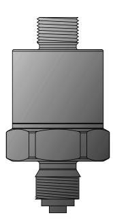
The **METPOINT**<sup>®</sup> pressure transducer of the PRM-SP series detects the relative pressure (gauge pressure) in **gaseous** and **liquid** media and transforms this measured value into a linear, pressure-proportional electrical output signal of 4 ... 20 mA or 0 ... 10 V.
