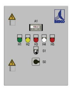
Temperature controller A1 S<sub>0</sub> Main switch S1 Starting switch H1 Converter operation / "Green" light H2 ALARM: Temperature monitor AUTO-RESET / "Yellow" light H3 ALARM: Safety temperature monitor AUTO-RESET / "RED" light H4 Reactor heating phase BEKOKAT® AUTO-RESET / "White" light H5 ALARM reactor min/max.
