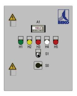
Α1 Temperature controller S0 Main switch S1 Starting switch H1 Converter operation / "Green" light H2 ALARM: Temperature monitor AUTO-RESET / "Yellow" light H3 ALARM: Safety temperature monitor AUTO-RESET / "RED" light H4 Reactor heating phase BEKOKAT® AUTO-RESET / "White" light ALARM reactor min/max. H5
